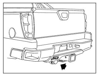
Your vehicle is equipped with the eight-wire trailer towing harness. This harness with a seven-pin universal heavy-duty trailer connector is attached to a bracket on the hitch platform.
